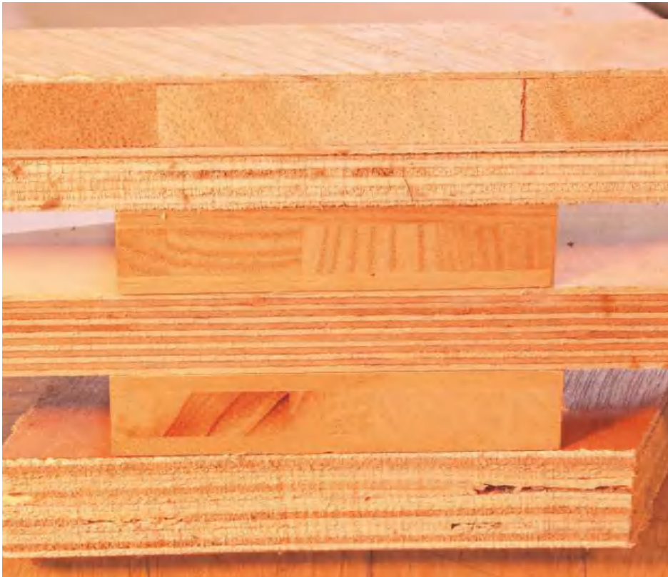
▲ Pic.1 Not all plywood is the same – look for thin lamins with no voids. The third and fourth ones down are the best quality. Decorative veneer facings are available at an extra cost
